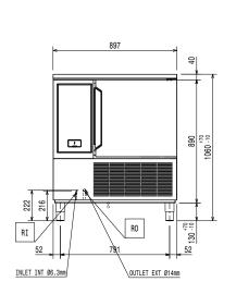
Drain Electrical inlet (power) ΕI Refrigerant Outlet
